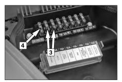
The ACC 1 / CLOCK and ACC 2 fuses [3] are designed for accessory equipment with a maximum current consumption of 10 amperes each. The respective connectors for this equipment are provided under the headlight cover. For more information, contact an authorized KTM workshop.
