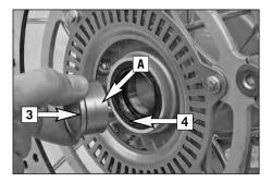
Before remounting the front wheel, clean and grease the shaft seal rings [4] and the bearing surface [A] of the distance bushings and mount the distance bushings (wide distance bushing in the left shaft seal ring). Slightly push back the brake pads with a screwdriver. Set up the front wheel facing in the running direction (see arrow [B] on the tire).
