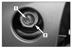
The adjusting screw [1] for the low-speed range can be adjusted with a screwdriver.
