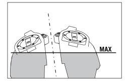
The 990 Adventure has 2 tanks with 1 filler cap each. Both filler caps can be locked and are equipped with a tank vent system. To open, insert the ignition key, turn 45° in a clockwise direction and fold up the filler cap. The ignition key can be pulled out to open the other filler cap. Simply press on the filler cap to close.
