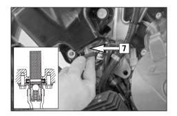
Carefully pull the oil screen [7] out of the oil tank.
