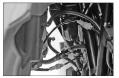
Mount the battery cover and tighten the screws to 25 Nm. Mount the lower screw on the right tank and tighten to 25 Nm.
