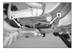
Mount the oil drain plug on the engine with a new seal ring and tighten to 20 Nm.
