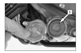
Insert a new oil filter [1] in the engine case, grease the O-ring and mount the oil filter cover together with the O-ring. Tighten the screws to 6 Nm.
