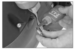
Apply Loctite 243 to the thread of the 4 screws, mount the underride protection and tighten the screws to 25 Nm.
